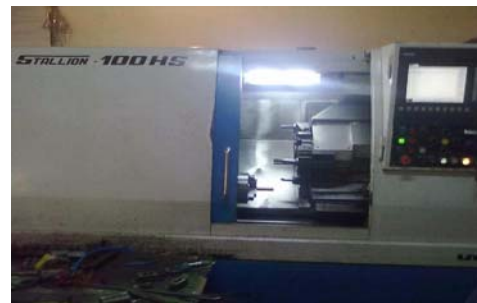
Fig. 2: HMT STALLION 100 HS CNC lathe
